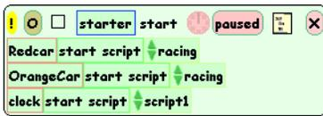
MouseDown on the **paused** button at the top of the script. Select “mouseUp” so that the script will run each time you release the mouse over the button.
